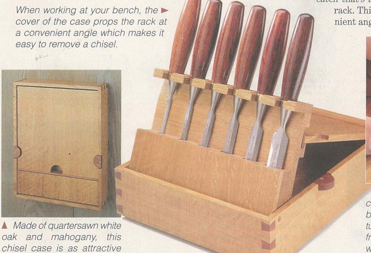
▲ To "unlock" the chisel case, simply rotate a turn-button on each side. The turnbuttons also keep the rack from tipping too far forward when the case is mounted on the wall, see photo above.
