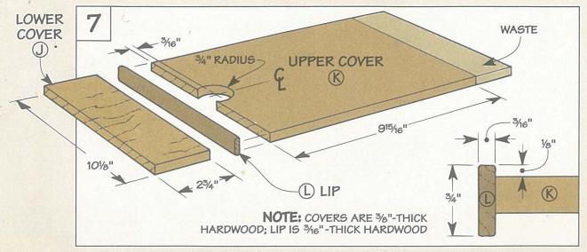
that's glued to the upper cover will hook into the catch on the back of the rack. (I used mahogany.)
