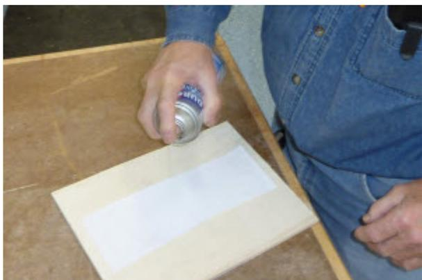
Start by creating your template. Cut out the attached pattern, and apply to 1/4" plywood or tempered hardboard using adhesive spray. Let the spray dry for about a minute before placing it on the template material, which will allow the paper pattern to be removed more easily.
