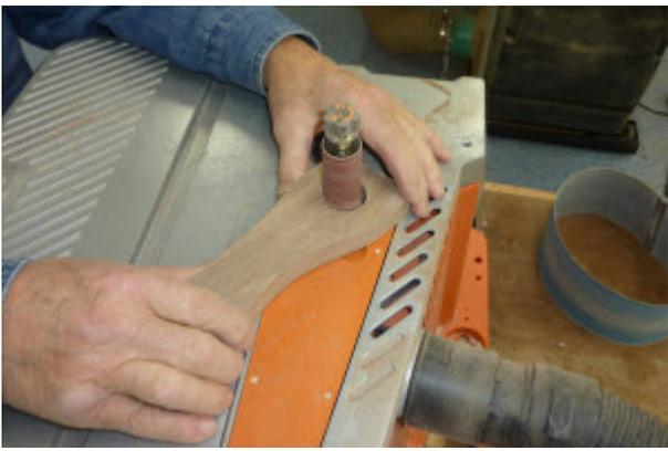
Use an oscillating spindle sander or other means to sand inside the holes. After all surfaces have been sanded using power equipment, hand sand to 400-grit to achieve a smooth feel.
