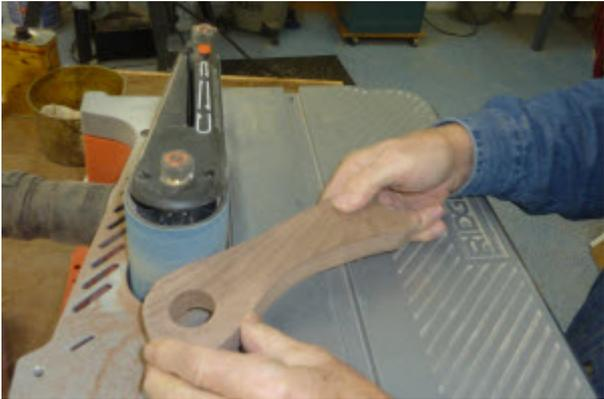
Sand to the line. Using a belt sander, carefully sand to the line for final shaping.
