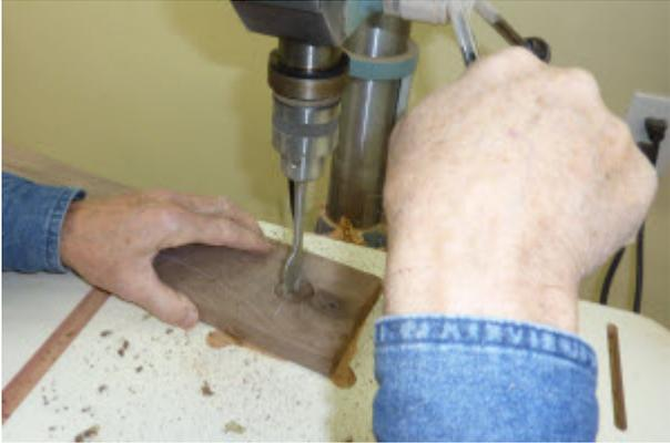
Drill holes. Use a 1-1/4" bit to drill holes as positioned in the template. The bottom contour could also be cut on the band saw, but given the tight radius we generally do this at the drill press, which provides a quick hole that is consistent in size with the top hole, and leaves a smooth surface that saves on sanding time later.
