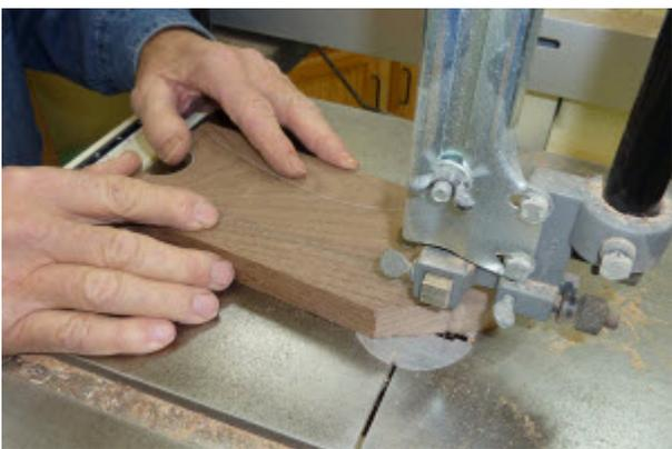
Cut rough shape on band saw. Using a band saw, cut the curved shapes, leaving the line for final shaping later.
