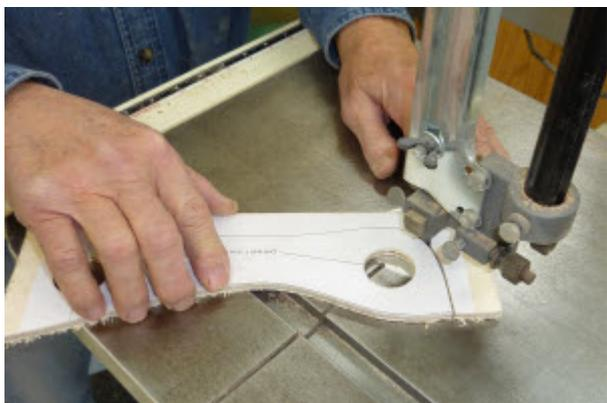
Cut out the template. First drill the 1-1/4" holes as indicated on the template. Then, use either a band saw or scroll saw to cut to the pattern lines, and sand the edges smooth.
