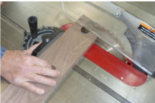
Cut the base angle. Prior to cutting the curved shape on the band saw, cut the base at a 35-degree angle.
