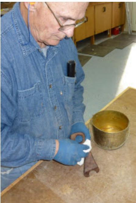
Finish using polyurethane or other durable finish. One way to support small pieces like this as the finish cures between coats is to tap some small finish nails about half way into a piece of scrap wood, leaving a bunch of nails sticking out a small amount at approximately the same height. This will support the piece without much contact surface area, allowing you to finish all sides in a single pass.
