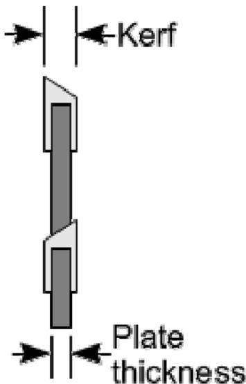
The "kerf" of a blade is the amount of material it removes from the stock, or, in other words, the width of the cutting teeth (and therefore, the cut). The saw plate thickness is less than that of the teeth, as can be seen in this diagram, which provides relief between the stock and the blade.
