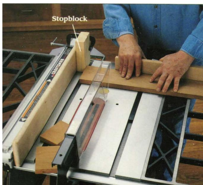
Note that the Stop Block must be clear of the end of the piece being cut before the leading edge of the piece contacts the blade. If this is not done then kickback **WILL** occur.
