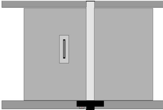
Here's a simplified view of the BT3 saw from above, showing the throat plate surrounding the blade, the fence assembly and the fence rails.
