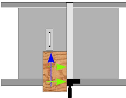
When feeding stock, ensure that it is held firmly against the fence by pressure in the direction of the fence (the green arrows). Once a good contact has been established with the fence, feeding can begin (blue arrow).
