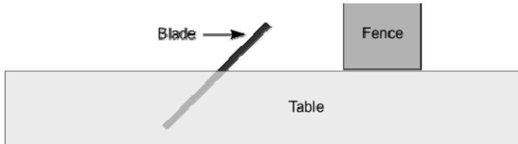
Move the fence to the left-hand side of the blade, like this:
